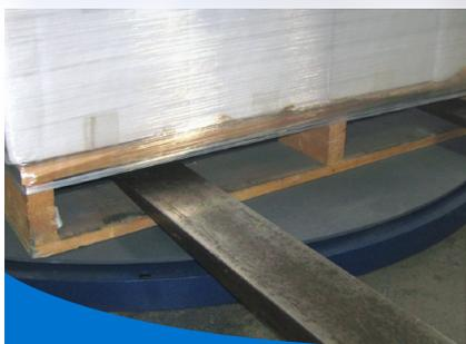
The cable is placed (*driven down*) just below the top boards of the pallet, low enough to lock the load yet high enough to avoid the forks from pallet jacks or lift trucks.
