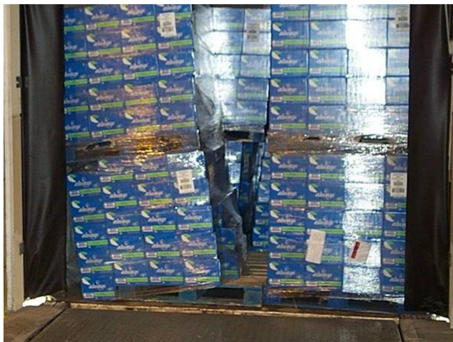
No Pallet Grip - film wrapped to bottom of pallet
