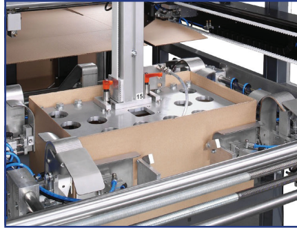
Square Tray Forming While the blank is being pressed through the forming unit by the stamp, the roll end tray tabs will be simultaneous rolled over and locked on all sides.
