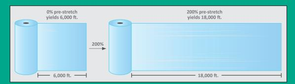
For example, at 100 percent pre-stretch, 6,000 ft. of film would turn into 12,000 ft. At 200 percent pre-stretch, 6,000 ft. of film would turn into 18,000 ft. of film, and so on. Little to no pre-stretch occurs when film i applied to the load by hand.
