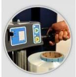
**Tension Control Knob** Turn tension knob clockwise to increase film tension, counterclockwise to reduce film tension.
