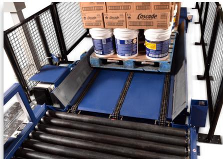
Guide rails help center the pallet on the conveyor.
