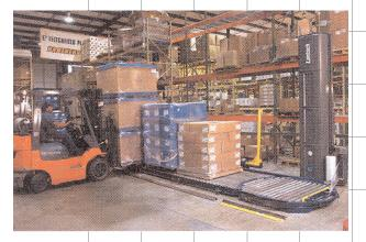
Accumulate wrapped loads on additional sections of gravity exit conveyor
