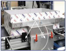
**Square Lid Application** While the lid is being applied by the folding unit, the tray is held in a square position by 2 brackets for accurate lid application.
