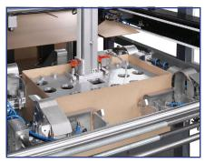
**Square Tray Forming**While the blank is being pressed through the forming unit by the stamp, the sides of the tray are simultaneous folded and glued on 4 sides.
