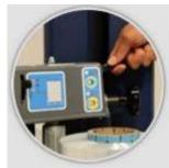
**Tension Lever** Turns film tension on and off for film threading and cycle
