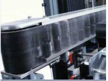
**CONTROLLED CASE TRANSPORT** Spring loaded side belts take over the case at the infeed side. The spring load functionality deals with tolerances in case width.
