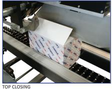
The side belts transport the case underneath special designed stainless steel curves. Due to the movement the long flaps close perfectly.
