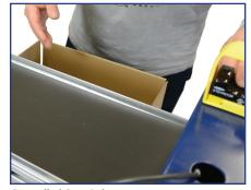
**Controlled Case Release** Once the case is loaded, the filled case is easily released to the case sealer infeed with the shutter release.
