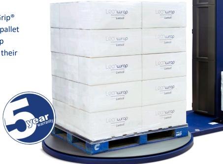
**Load Guardian** is Lantech's patented control system that *creates, maintains* and *delivers* the right containment force for safe-to-ship loads every time. It minimizes operator interaction and eliminates the guess work for stretch wrapping any load configuration.
