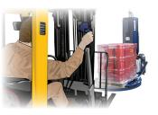
Click-n-Go remote meets the latest safety requirements outlined by the National Electrical Code. Using infrared technology and two-step activation process, the Click-n-Go is immune to accidental activation from stray radio frequency.
