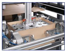
**Square Tray Forming**While the blank is being pressed through the forming unit by the stamp, the sides of the tray are simultaneous folded and glued on 4 sides.
